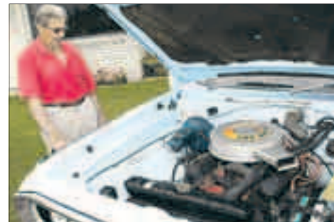
V8 FAN: Lloyd was keen to make sure I knew this was the 360ci — Chrysler's biggest V8 available in New Zealand at the time.
